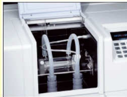
Figure 2. Sample compartment for the Series 341/343 Polarimeters with standard cell, temperature probe with conveniently removable thermostating tubing.
