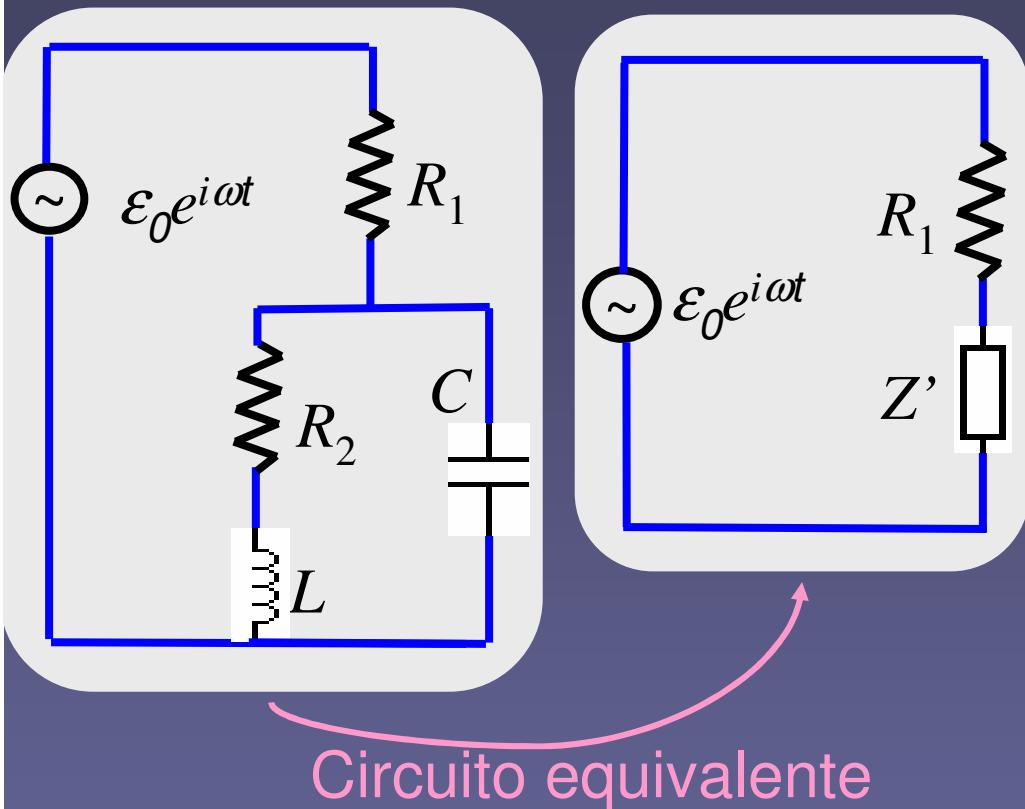
$$\begin{aligned}\frac{1}{Z'} &= \frac{1}{1/i\omega C} + \frac{1}{R_2 + i\omega L} \\ &= i\omega C + \frac{1}{R_2 + i\omega L} \\ &= \frac{(R_2 + i\omega L)i\omega C + 1}{R_2 + i\omega L}\end{aligned}$$
