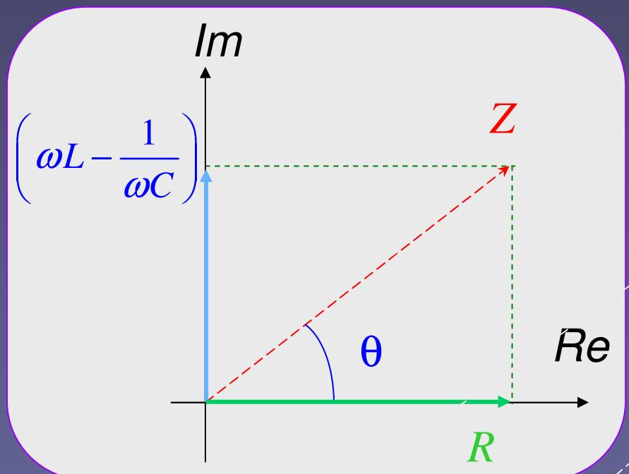
$$\begin{aligned} |Z| &= \sqrt{R^2 + \left( \omega L - \frac{1}{\omega C} \right)^2} \\ \cos \theta &= \frac{R}{|Z|} \\ \sin \theta &= \frac{1}{|Z|} \left( \omega L - \frac{1}{\omega C} \right) \end{aligned}$$
